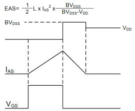
Figure 11. Unclamped Inductive Switching
