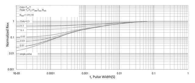
Figure 9. Normalized Maximum Transient Thermal Impedance
